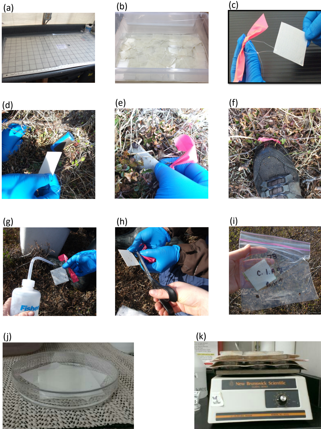
Fig. S1 Procedures for IEM preparation, incubation, retrieval, and elution. (a): Measure out 5 cm x 5 cm sections and cut them out with a clean knife while the IEM sheet is still in its plastic covering. (b): Soak the IEM squares in the charging solution. (c): Tag one corner of each IEM with a plastic cloth barb and flagging tape. (d): Cut a vertical slit in the soil to the specific depth. (e): Insert the IEM down into the slit until it reaches the chosen depth. (f): Pack down the soil on either side to secure the IEM. (g): Rinse the IEM with distilled water. (h): Cut off the cloth barb and flagging tap from the IEM. (i): Store the IEM in a pre-labelled clean bag. (j) Place the multiple IEM squares from within the same replicate sampling area in a Petri dish and fill with elution solution to cover them. (k): Place the Petri dishes securely on the shaker table and shake for 2h.
