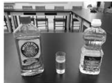
Less dense cooking oil floats on top of the more dense liquid soap.
