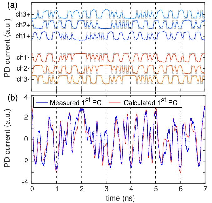
Fig. 2. Example of a PCA task on a 13 Gbaud bit pattern yielding 93% accuracy (cf. caption of Fig. 3). (a) The modulated waveforms before the weight bank (Fig. 1.(3)). Note the delay of 1 ns between subsequent channels. The distortion from the MC bit pattern (gray) arises from the bandwidth limitation in the PPG circuit. (b) After completion of PCA task, the measured first PC waveform (Fig. 1.(4)) is compared to the SVD-calculated one.
