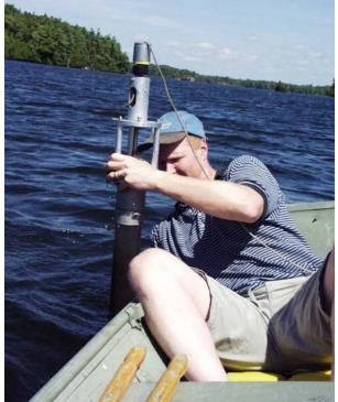
Holding bottom of core tube and plug to prevent plug from falling out (which would lead to lost sediment), lift corer slowly out of water.
