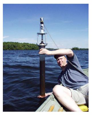
Be careful not to disturb sedimentwater interface.
