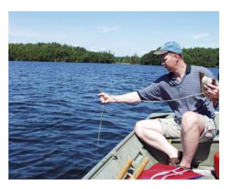
Slowly lower corer into water. Lower slowly until corer penetrates into sediment (max. speed =~ 0.5m/sec). It is important not to let the corer freefall, as this can " blow away" surface sediments.
