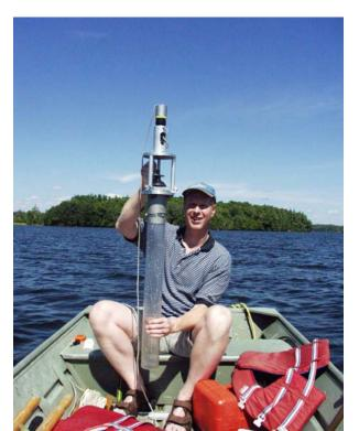
Attach core tube to corer. Make sure flat end of corer is square against ring seal. Tighten hose clamp on tube housing using nut driver, do not over tighten. Core tube should not move within the housing.
