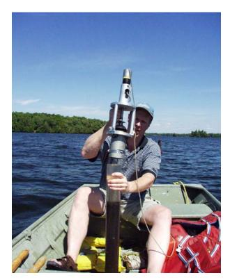
Ensuring the core is secured, loosen hose clamp securing core tube to corer, and remove corer form core. Be careful not to disturb core.
