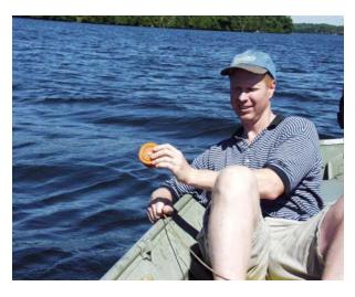
While core tube is submerged, insert core plug (black rubber or orange bung) to form a seal in bottom of corer.
