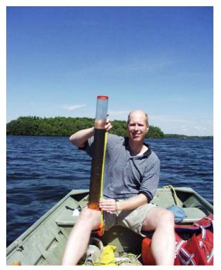
Add cap to top of core. Secure plug at bottom of core tube with electrical tape to prevent plug from accidentally slipping. Label core tube with masking tape and permanent ink. (lake name, core, top/bottom, date).
