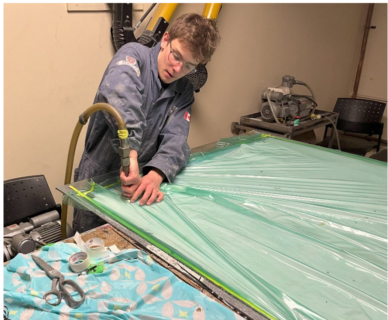
Blair working with the Queen’s Formula SAE Racing Team. He is vacuum sealing a composite sandwich panel to cure under vacuum pressure. The panel is to be water jetted and used in the aerodynamics’ assembly.
