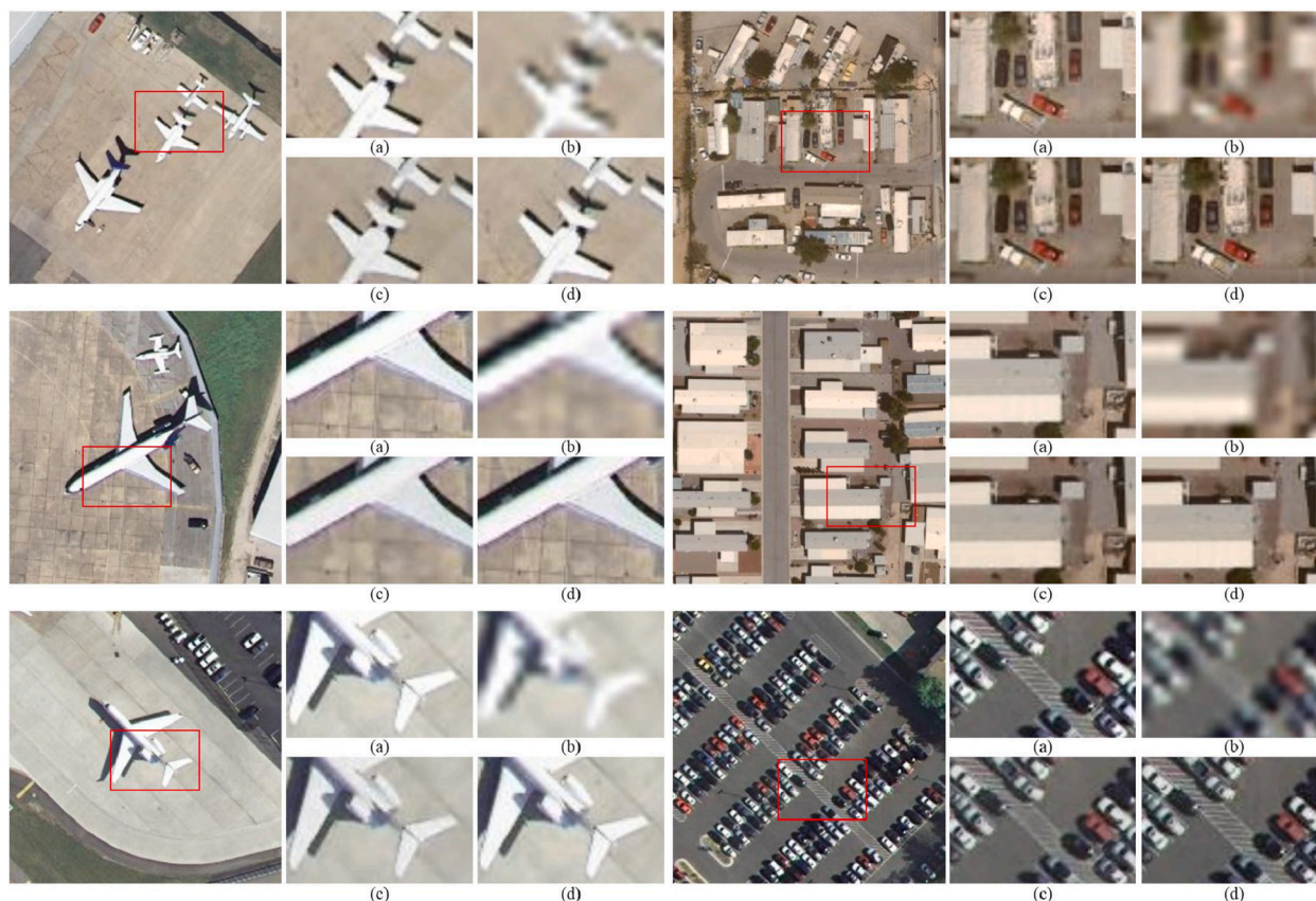
Fig. 12. Super-resolution results presented in Yu et al. (2020): (a) HR, (b) bicubic resampling, (c) SRFeat (Park et al., 2018), (d) E-DBPN (Yu et al., 2020).
