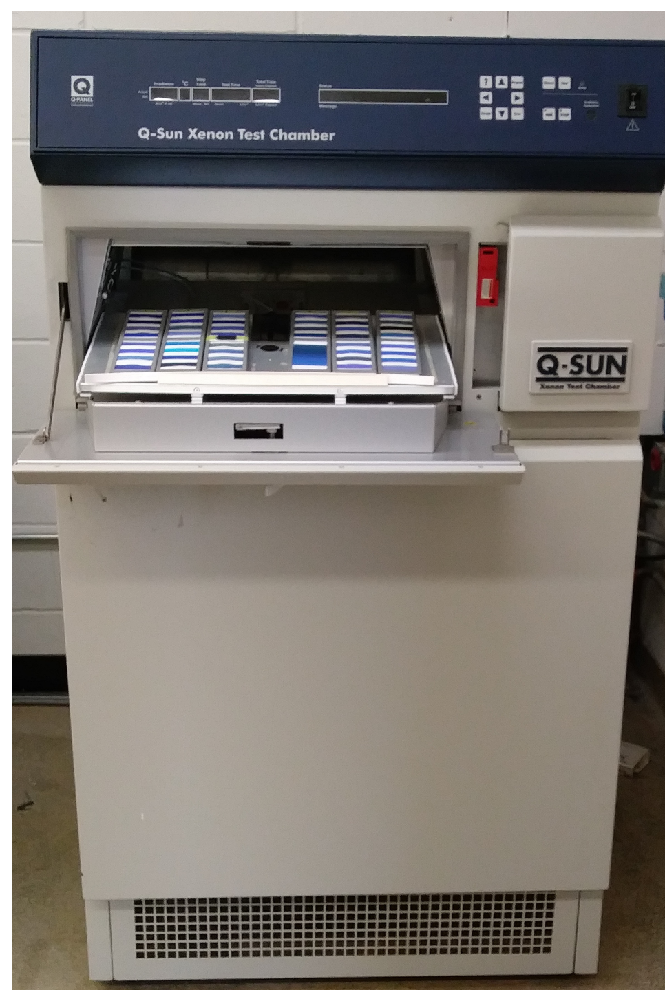
Samples in the Q-Sun Xenon Chamber at Queen's University.
