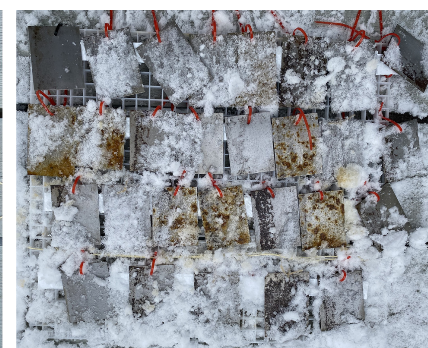
Fig. 4: Coupons in aging setup during aging, showing start of rust formation in snow
