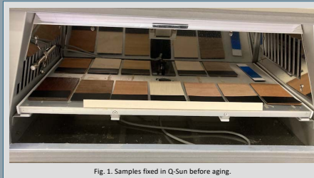
Fig. 1. Samples fixed in Q-Sun before aging.
