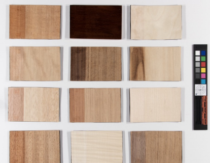
Fig. 4. Samples after aging. Left side, covered during aging, shows colour change.
