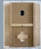
Fig. 2. Jig used to take repeated spectrophotometer measurements. Courtesy of Anne-Stéphanie Etienne.
