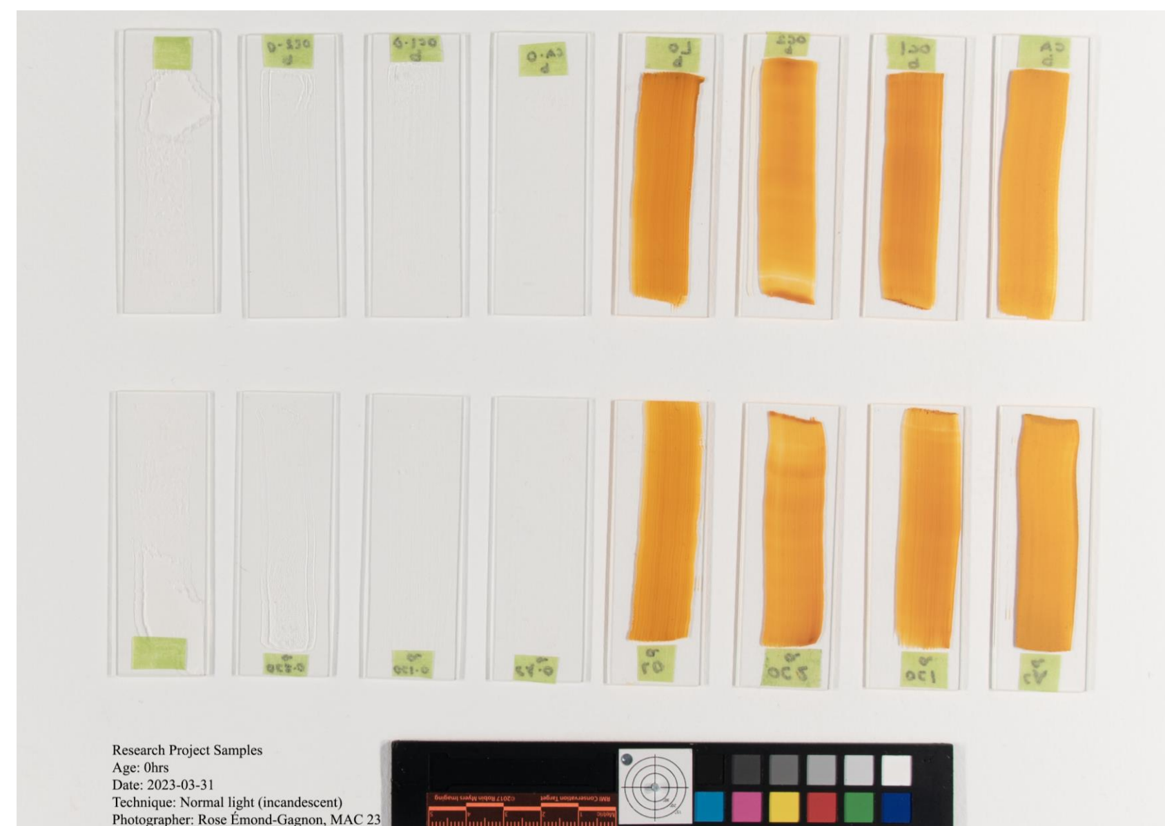
Figure 1 (top). Paint films and controls before ageing. Table 1 (left). Formulations of paint films and controls.
