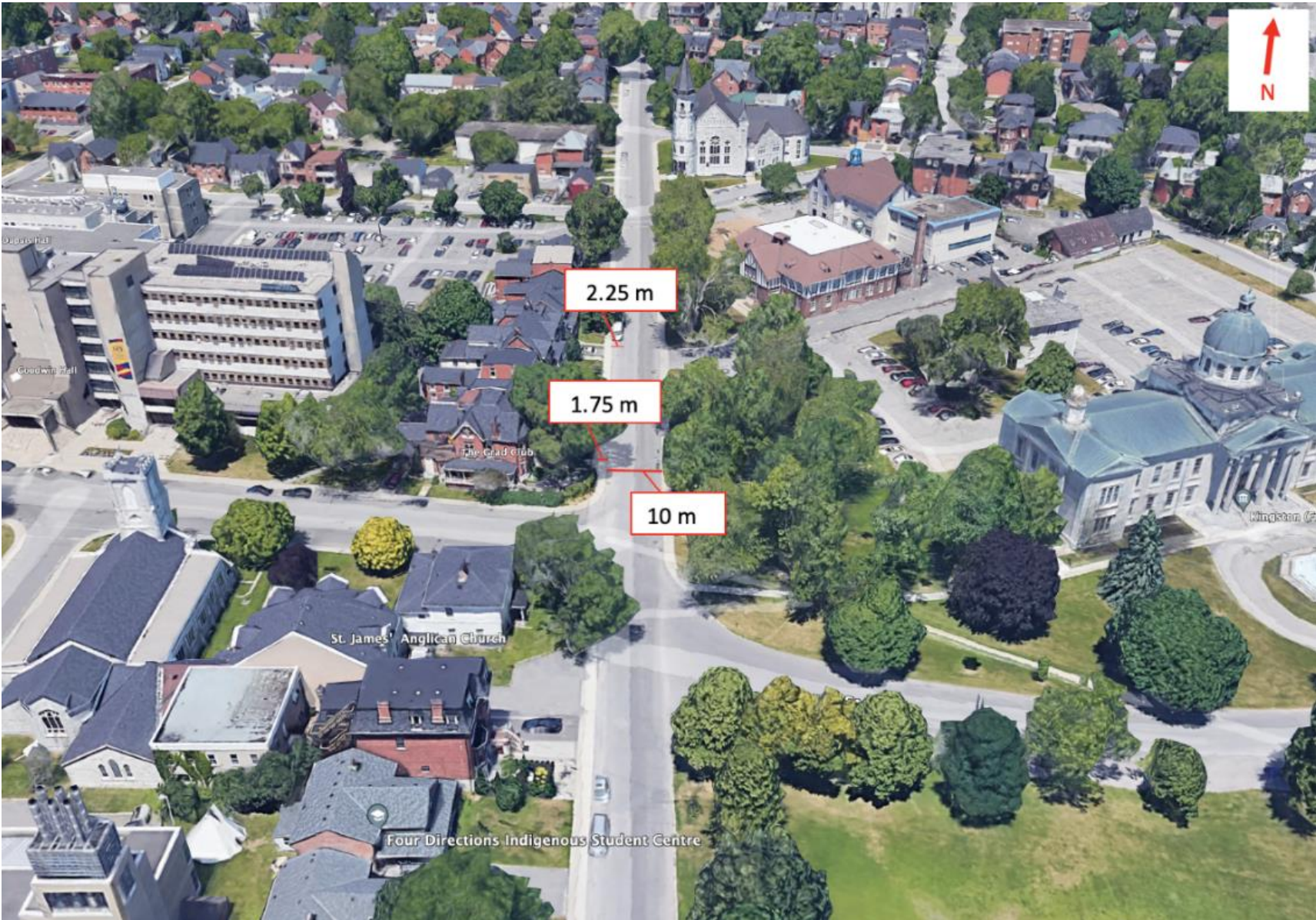
Figure 45: Current Cross-section Dimensions for Barrie St. (Sidewalks are the same dimension on both sides) (Google Earth 2022d)
