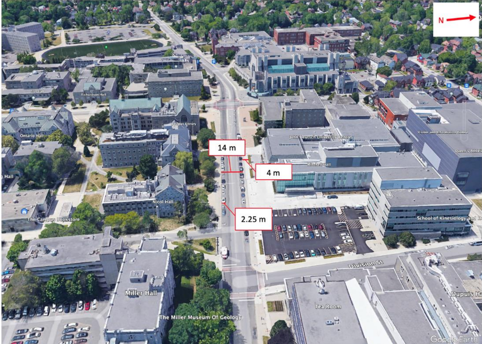
Figure 43: Current Cross-section Dimensions for Union St. (Sidewalks are the same dimension on both sides) (Google Earth 2022b)
