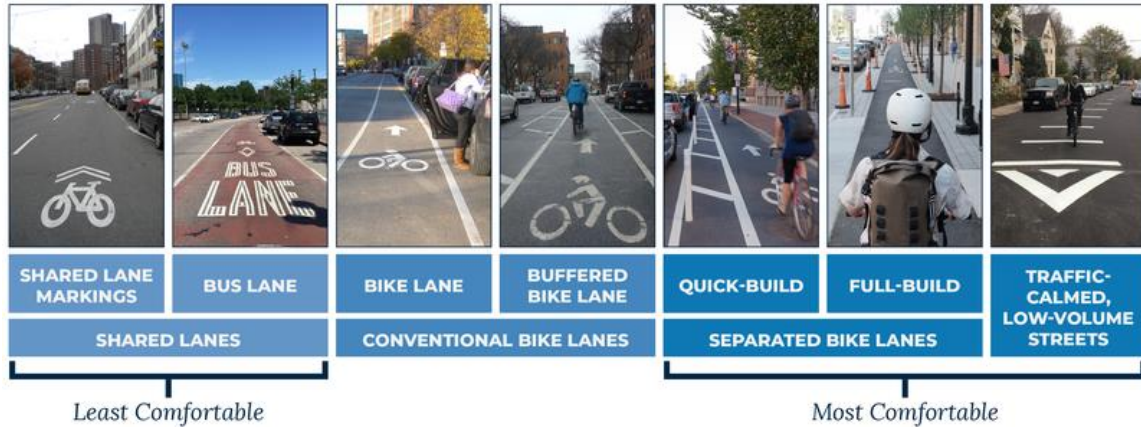
Figure 7: Different Types of Bike Lanes Used in Transportation Planning and Design (City of Boston 2016)
