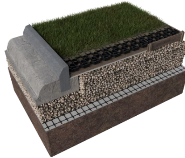
Figure 7-2 Examples of possible driveable greening infrastructure that utilizes structural load bearing components below grade, allowing vegetation to grow unobstructed at the surface.
