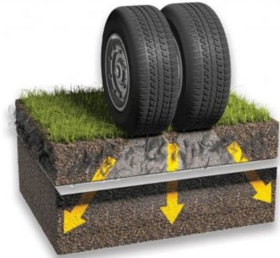
Figure 7-2 Examples of possible driveable greening infrastructure that utilizes structural load bearing components below grade, allowing vegetation to grow unobstructed at the surface.
