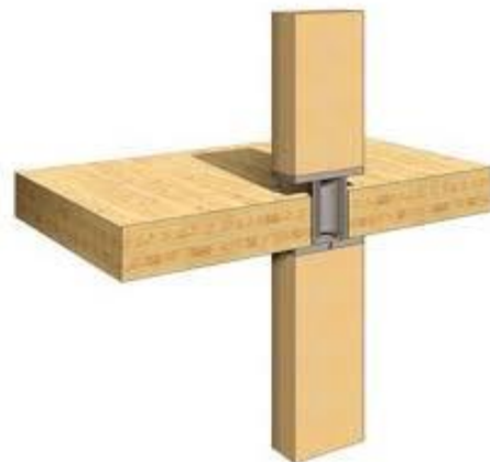
FIGURE 10: CROSS-SECTION OF THE COLUMN TO COLUMN CONNECTION IN THE BROCK COMMONS BUILDING (NATURALLY WOOD 2016B)
