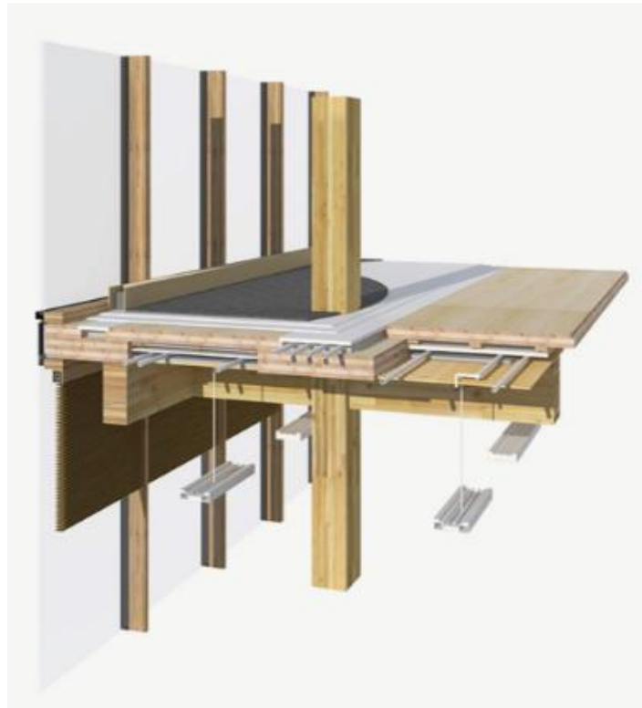
FIGURE 26: STRUCTURAL ELEMENTS IN THE FLOOR SYSTEM IN THE WIDC (MICHAEL GREEN ARCHITECTURE 2014)
