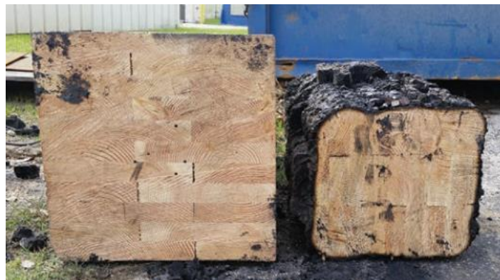
FIGURE 7: BEFORE AND AFTER EFFECTS OF THE CHAR LAYER FOR A GLULAM COLUMN (MCLAIN AND BRENEMAN 2021).
