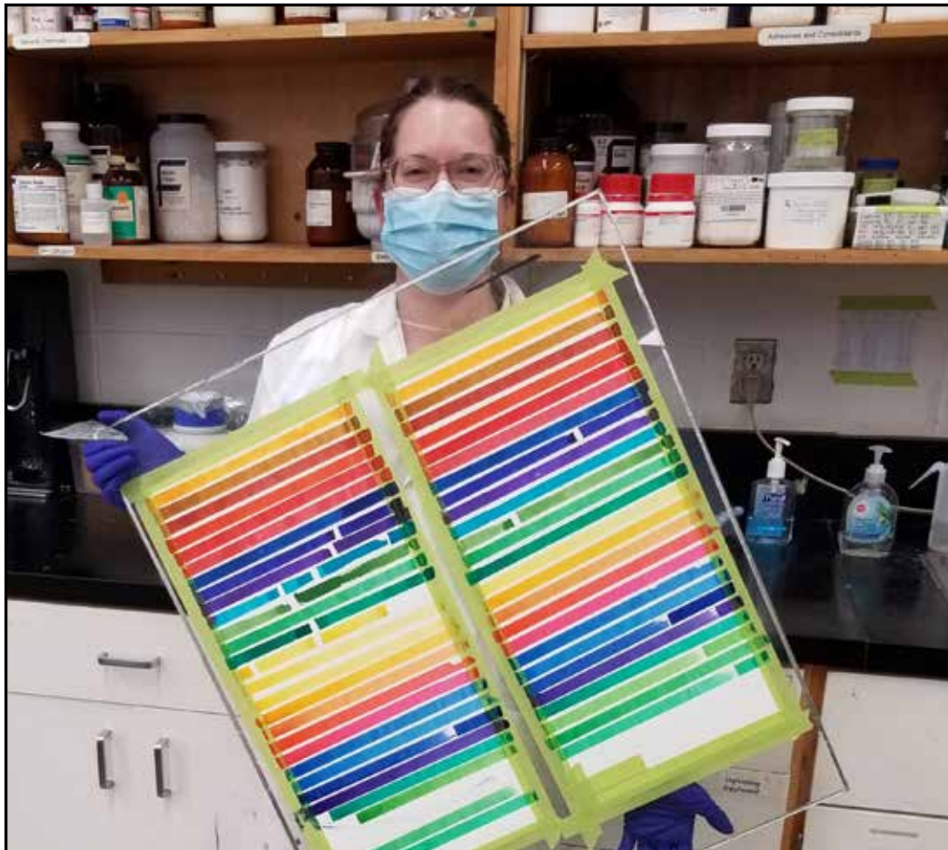
Sandrine Blais (MAC'22) showing off her final ink samples for her research project, which studies the lightfastness of modern dye-based inks on paper.
